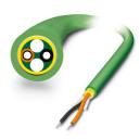
POF PROFINET installation cable for assembly (IP20 heads only) for installation in stationary systems and machines, individual elements of polyamide (PA), halogen-free, ozone- and UV-resistant, with reinforced polyurethane (PUR) outer sheath
