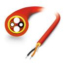
Robust POF installation cable for assembly (IP20 heads only) for installation in stationary systems and machines with individual elements made of polyamide (PA), halogen-free, ozone and UV resistant, with reinforced polyurethane (PUR) outer sheath
