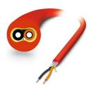
POF installation cable for assembly (IP20 heads only) for installation in stationary systems and machines with individual elements made of polyamide (PA), halogen-free, ozone and UV resistant, with a polyurethane (PUR) outer sheath
