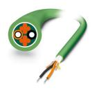
Highly flexible POF PROFINET cable (IP20 heads only) for use in drag chains. Individual elements made from extremely wear-resistant polyamide (PA). The cable is halogen-free, ozone and UV resistant, and has a rugged polyurethane (PUR) outer sheath.
