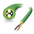
PROFINET polymer fiber cable, duplex 980  $\mu$ m/1000  $\mu$ m, heavy-weight design, for installation in stationary systems and machines, by the meter, without male connector
